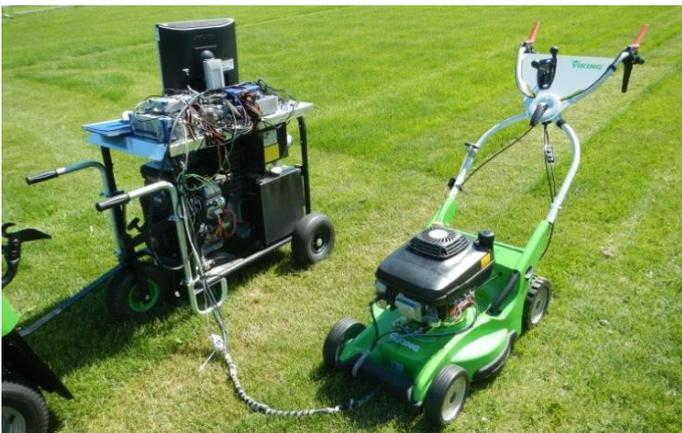
**Figure 7: Measurement setup of the lawnmower for the real world tests**
