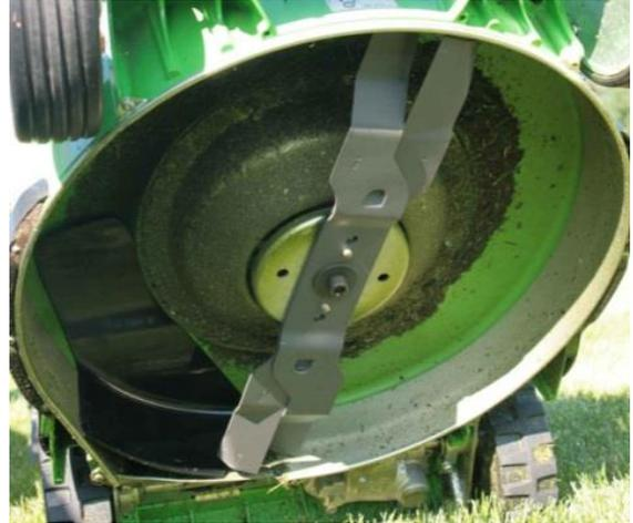
**Figure 12: Mulching blade in lawnmower**
