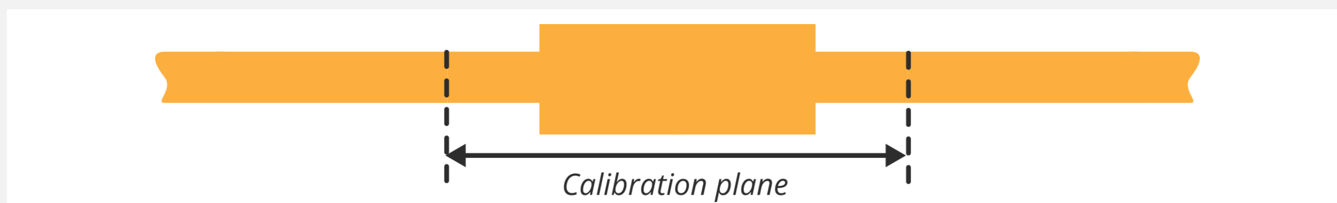
Fig. 3: Illustration of stepped impedance line (Beatty line).
