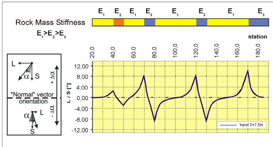
Figure 2. Variation of displacement vector orientation when tunnelling in a heterogeneous rock mass, result of numerical simulation
