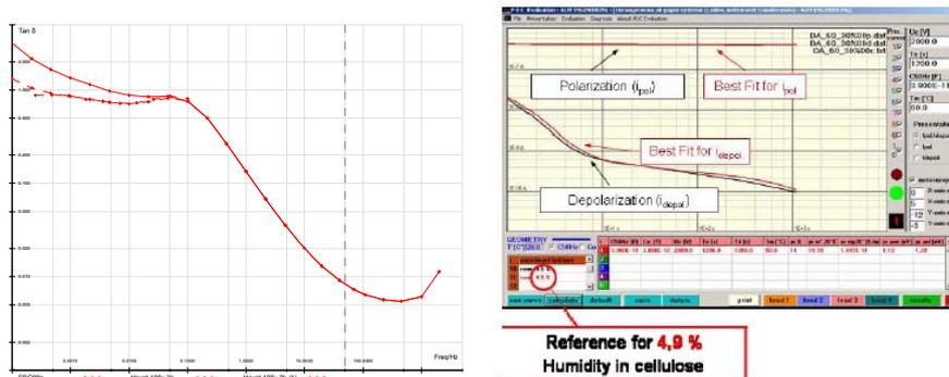
Figure 2 - Results of FDS and PDC Analysis
