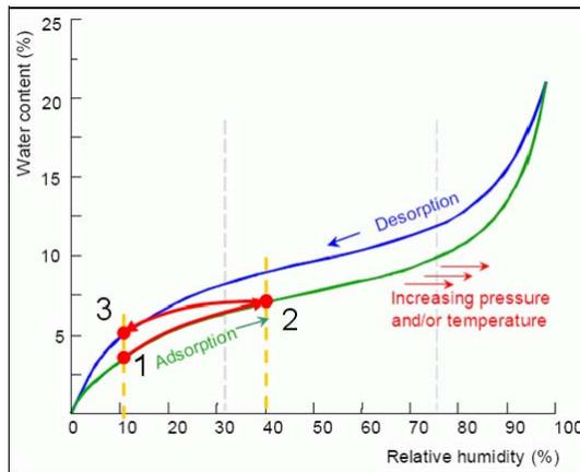
Figure 3 - Adsorption and desorption isotherm for cellulose [2]
