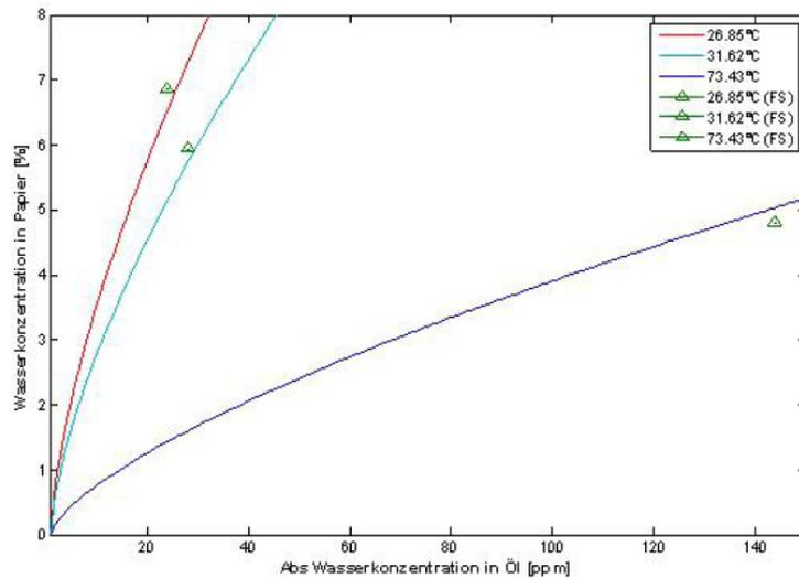
Figure 5 - Relative moisture in cellulose and oil calculated and measured with Karl-Fischer-Titration [6]
