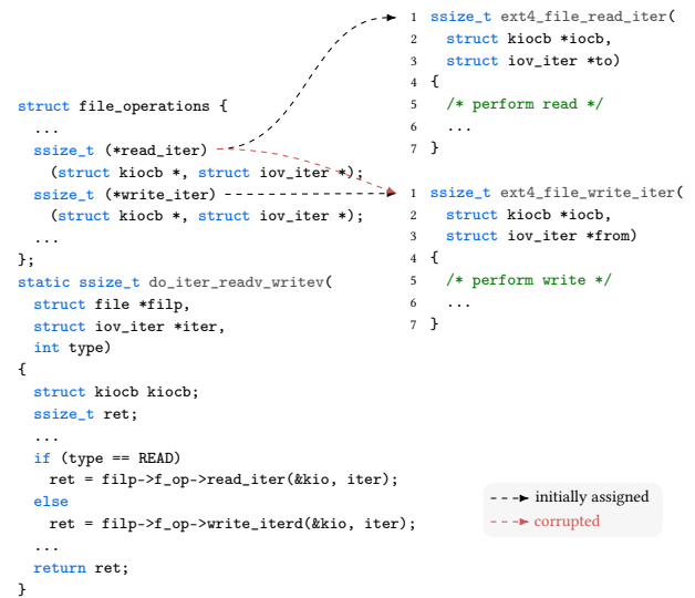
Figure 10: Exploitation to break signature-granular CFI. By overwriting the function pointer read_iter with ext4_file_write_iter an attacker enforces to call the write function on a read request.
