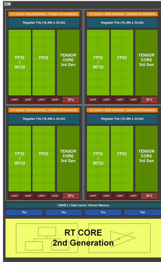
Figure 2.2: Nvidia Ampere GA102 streaming multiprocessor [37]. Threadblocks with up to 1024 threads are scheduled on a single streaming multiprocessor. Each streaming multiprocessor consists of 4 processing units. Warps with 32 threads are executed in parallel on each processing unit.
